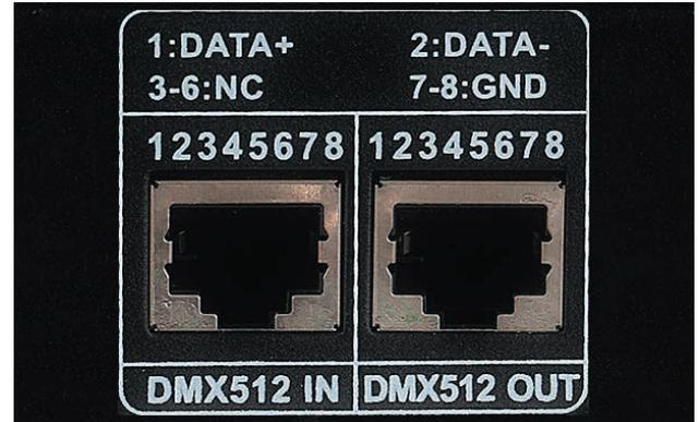
Uses RJ45 as interface signal.
